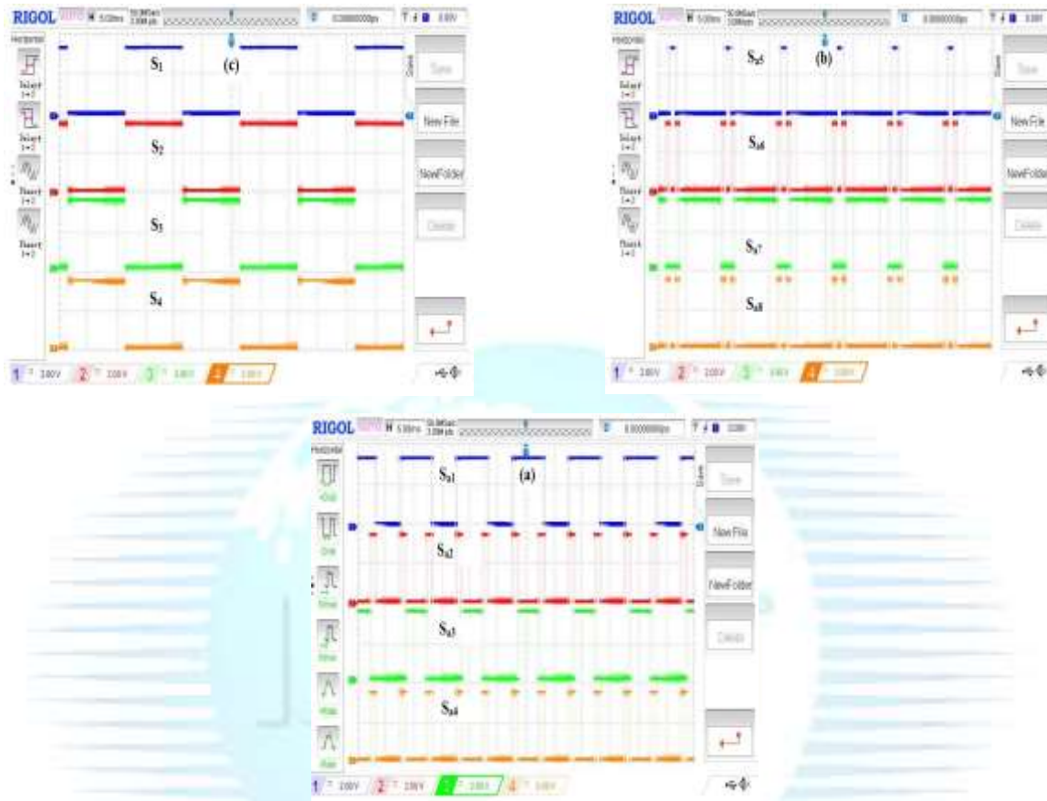
Figure 13 Switching pulses for Phase A using PD ISCPWM (a) Cell 1 (b) Cell 2 (c) H-Bridge
